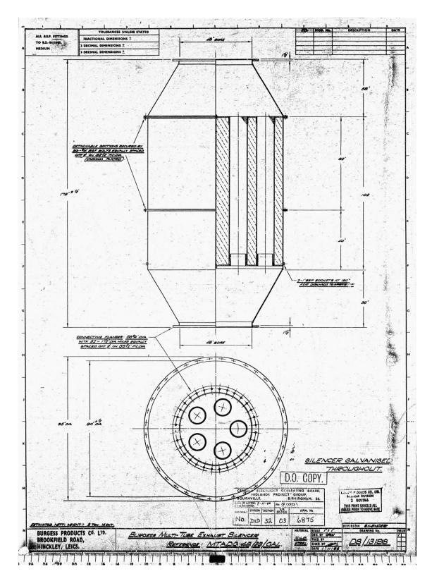
In 2002 an analysis of routine water condensate samples taken from the clean steam drain indicated slightly raised silicate concentrations. It was deduced that the source of the silicate was erosion of the pitted surface of the A-glass packing within the silencers, the result of repeated scouring of the glass fibre twice daily by superheated steam.
